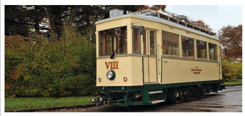
Three of the old railcars were converted to the new 900 mm track gauge and equipped with newest technologies in the course of the Pöstlingbergbahn reconstruction project.
